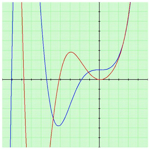
The blue line is the Kappa<sub>3</sub> function and the red line is its first derivative. When x is positive, the functions look very much like the hyperbolic trig functions but for x negative, they oscillate with ever increasing amplitude.
