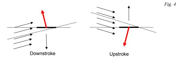
(It is equally clear that, on average, this wing will generate no lift – but that is because the angle of attack is zero. I have, for simplicity omitted the induced drag here. We shall consider the drag forces later. All that we require is that there shall be a net *forward* component of the lift.)
