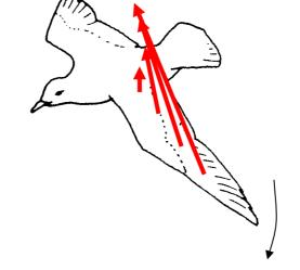
As we move from the shoulder to the wing, the lift increases in size and inclines more and more forward. Since the angle of attack at the wingtip is equal to the Strouhal angle, the angle of attack  $\alpha$  at a distance *r* from the wing root is
