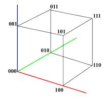
Fig 2: Configuration space of a 3-colour LED
