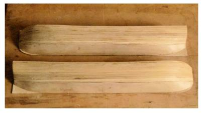
The final task is to glue the two halves of the hull together.
